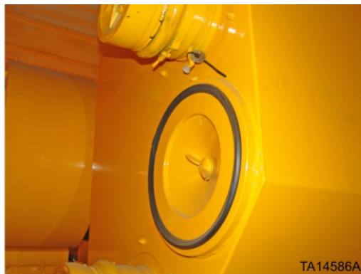
Figure 110. Engine safety inner and outer filter cover
