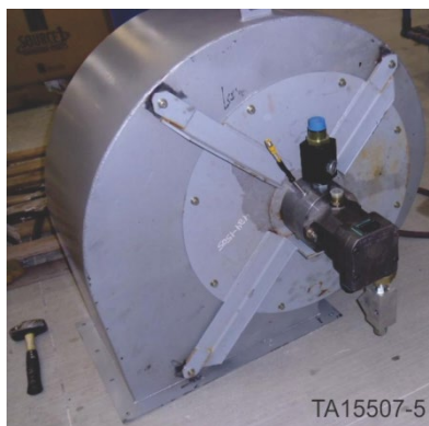
Figure 51. Blower removed and placed in work area
