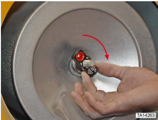
Figure 119. Installation of engine safety filter retaining nut
