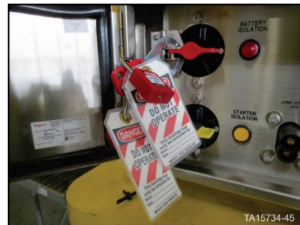
Figure 44. GEN 2 Battery Isolation Box – Battery isolation switch in OFF position with locks in place
