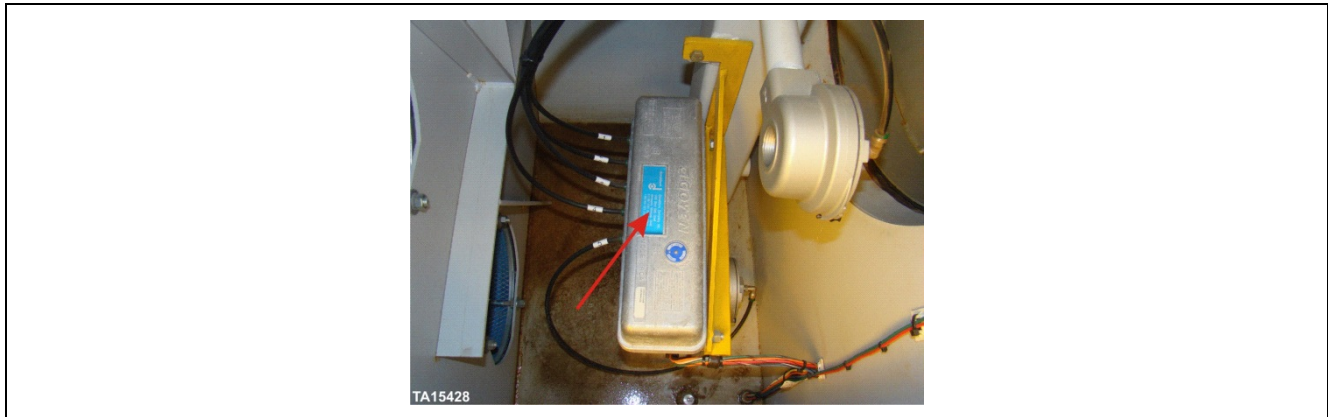
Figure 17. Solenoid enclosure-solenoid valves-mounting position
