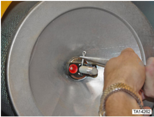
Figure 114. Removal of cotter pin from engine secondary (safety) filter indicator wing nut
