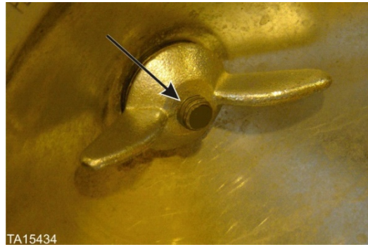
Two to three threads typically extend through the wing nut
