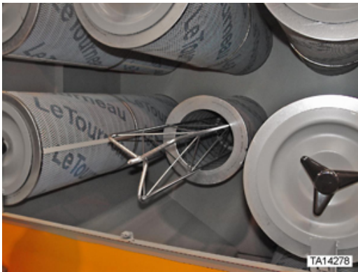
Figure 105. View of inner “KLENZ™” filter installed with gasket against flange at rear of filter chamber
