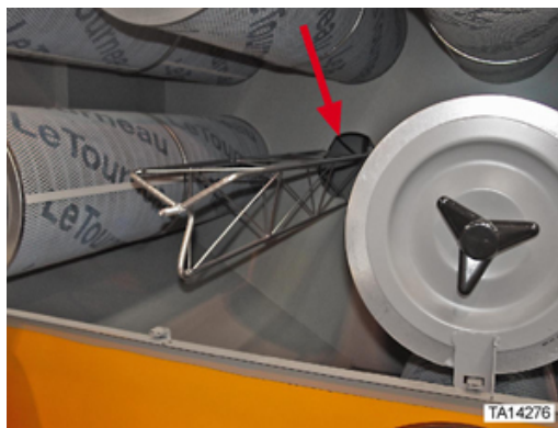
Figure 98. “KLENZ™” filters support racking flange at rear of filter chamber that filters must seal against
