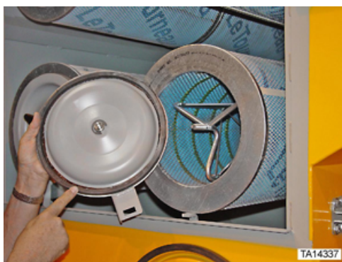
Figure 99. Inspection of tabbed cover gasket
