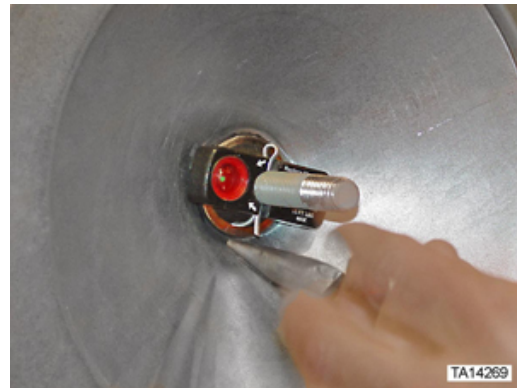
Figure 120. Installation of cotter pin to retaining nut
