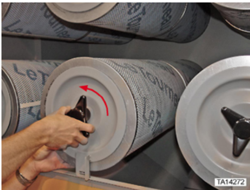
Figure 96. Removal of “KLENZ™” filter tabbed cover
