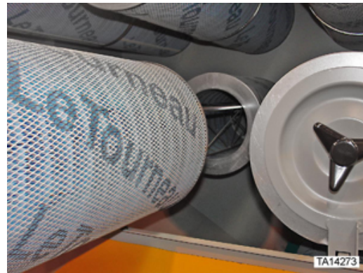
Figure 106. Installation of outer “KLENZ™” Filter
