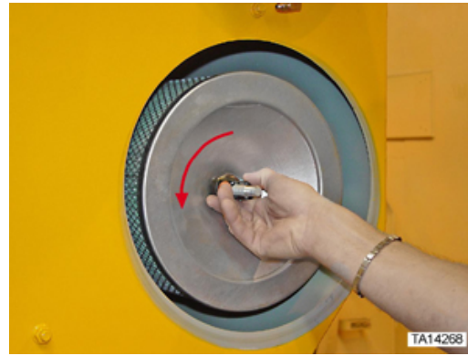
Figure 115. Removal of engine secondary (safety) filter indicator wing nut
