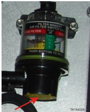
Reset button Internal indicator with no restriction shown
