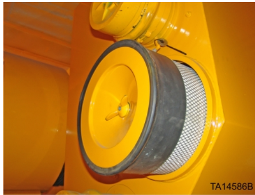
Figure 111. Engine safety outer filter rubber sleeve
