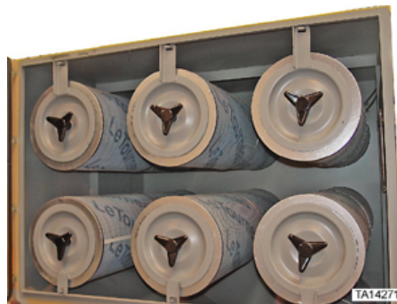
Figure 85. View inside typical filter chambers (number of filters might vary by machine model)
