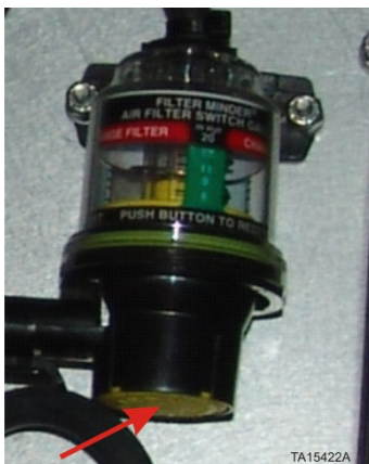
Figure 25. Reset button located on bottom of restriction gauge
