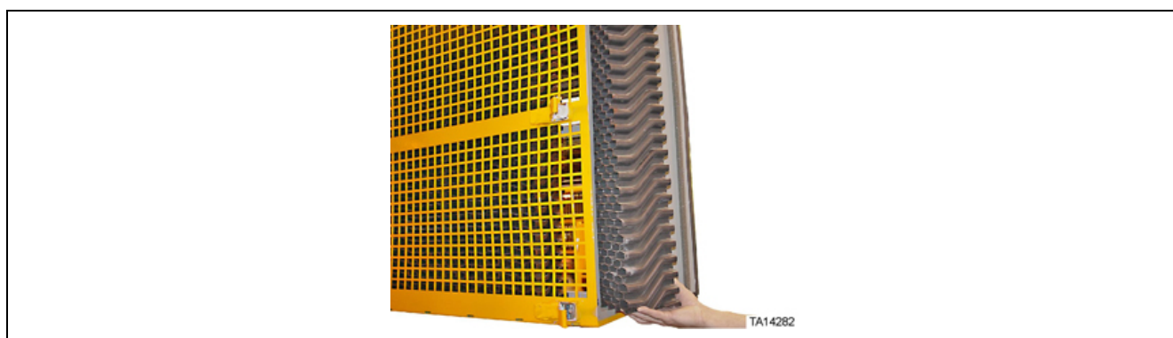
Figure 79. Mist eliminator panel
