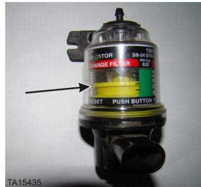
The internal indicator is shown with about 1/2 restriction indicated
