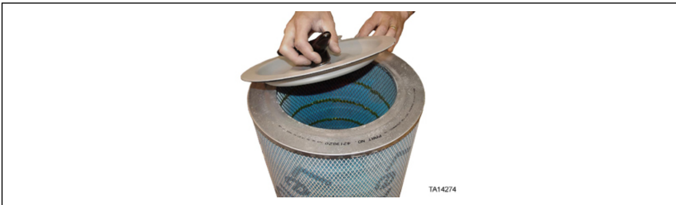
Figure 100. Check tabbed cover for warpage by placing against mating surface of new filter
