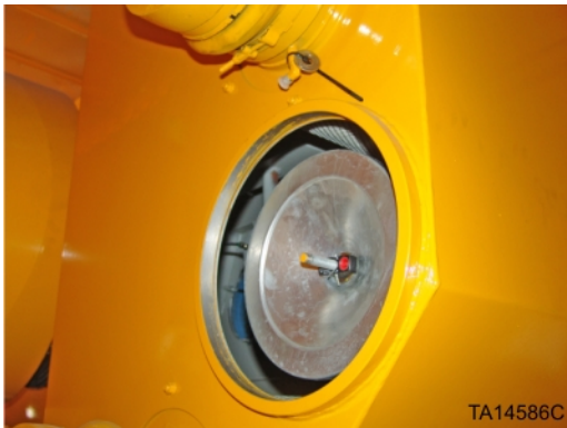
Figure 112. Inner 8" (203 mm) secondary (safety) filter element with indicator wing nut
