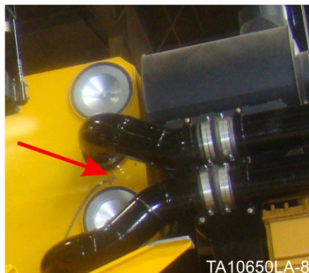
Figure 26. Engine filter safety adapter location
