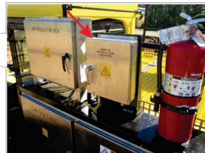
Figure 24. Engine filter restriction gauge location
