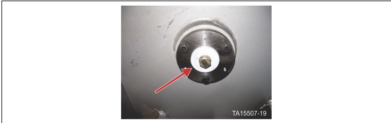
Figure 58. Blower wheel bushing capture bolt
